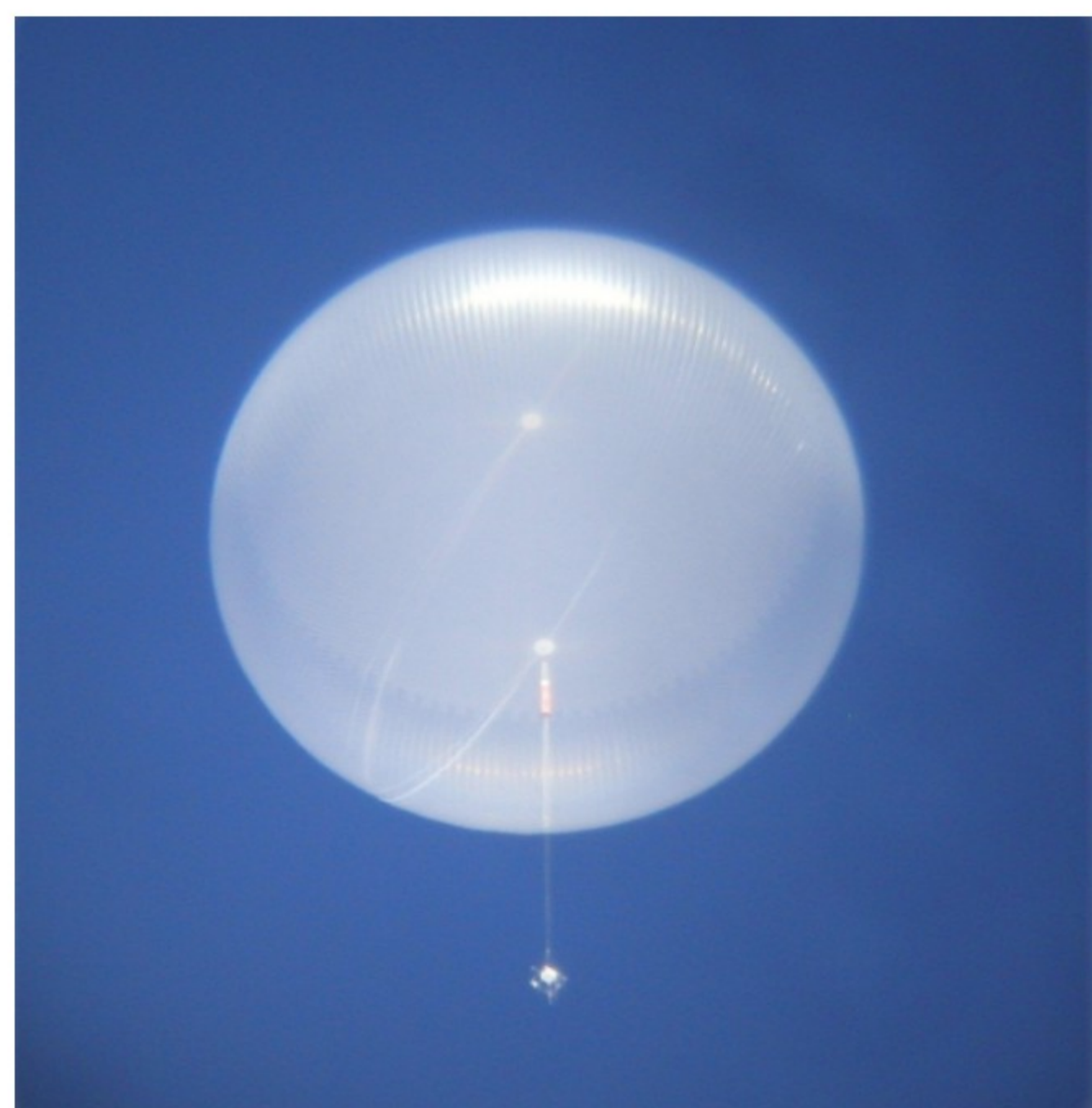
The super pressure balloon is at the cutting edge of NASA's stratospheric balloon program. They can hoist payloads of nearly 5000 pounds to heights above 120,000 feet. Unlike their older "zero-pressure" siblings, super pressure balloons are sealed, enabling them to remain aloft for over a month at a relatively stable altitude. Development began roughly a decade ago on the super pressure balloons, which expand to the size of a football stadium. (Courtesy Photo)
