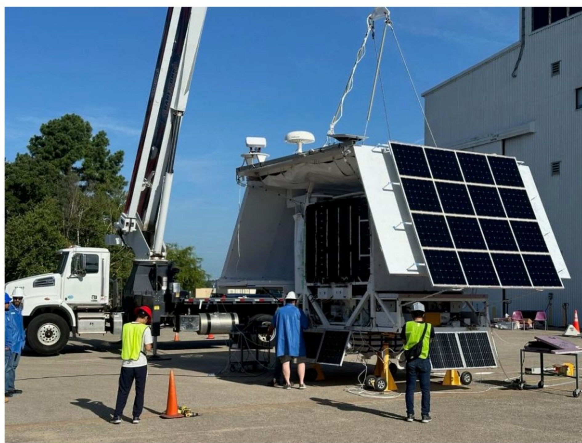
GAPS (the General Antiparticle Spectrometer) gets rigged and integrated in Palestine at the Columbia Scientific Balloon Facility. (NASA/Courtesy Photo)
